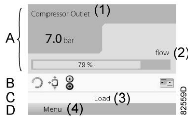
Typical Main screen (2 value lines), compressors with frequency converter
