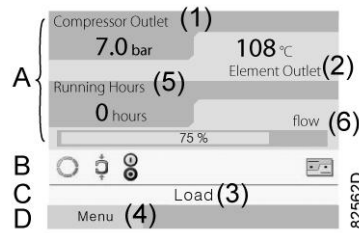
Typical Main screen (4 value lines), compressors with frequency converter
