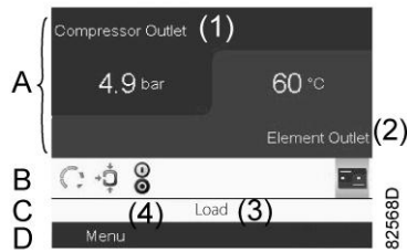
Typical Main screen (2 value lines), fixed speed compressors
