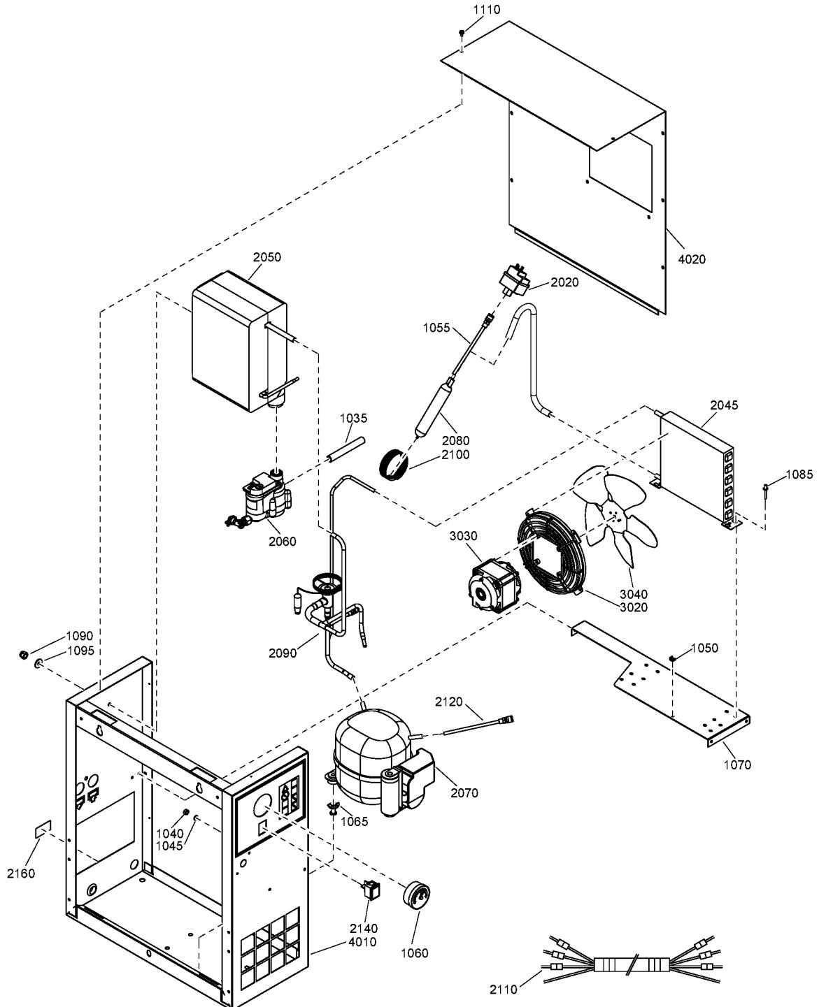
**32 - Air dryer components QRS 15, QRSM 20 - TRI-V- 575V/60Hz - CRNASME - UL-
