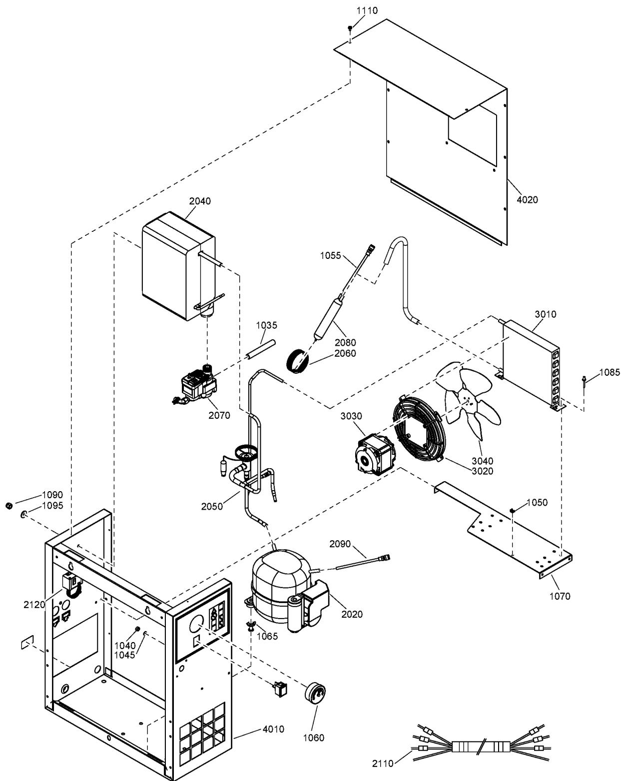
**34 - Air dryer components CPM 15, CPM 20 - 400V/50Hz - AS1210 - IEC - With 1 time size integrated dryer**
