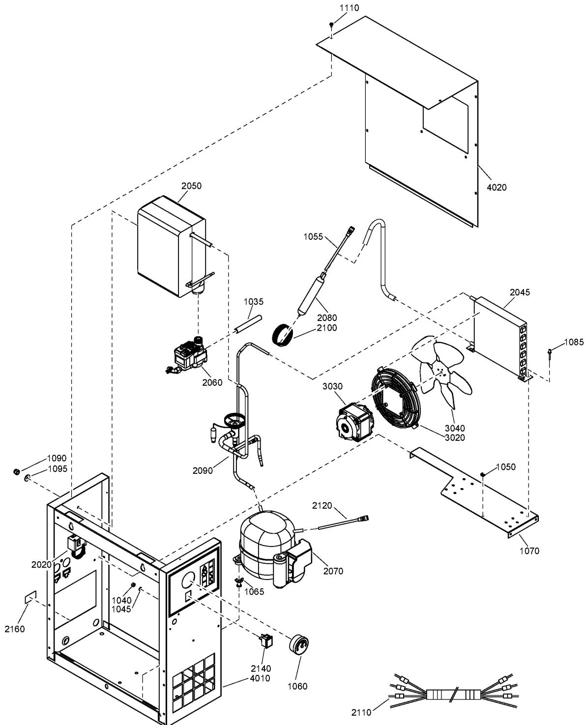
**33 - Air dryer components QRS 15, QRSM 20 - TRI-V- 575V/60Hz - CRNASME - UL-
