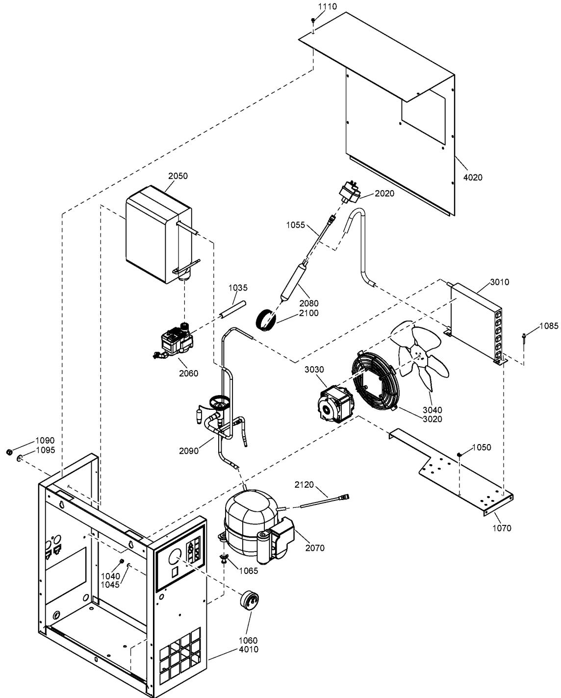
**20 - Air dryer components CPM 15, CPM 20 - (230V/50Hz - CE, 400V/50Hz - AS1210, CE, MOM, SAASME) - IEC - Without integrated dryer size, CPM 10 - 400V/50Hz - IEC - With 1 time size integrated dryer (11/10/2016 - 07/11/2018)**
