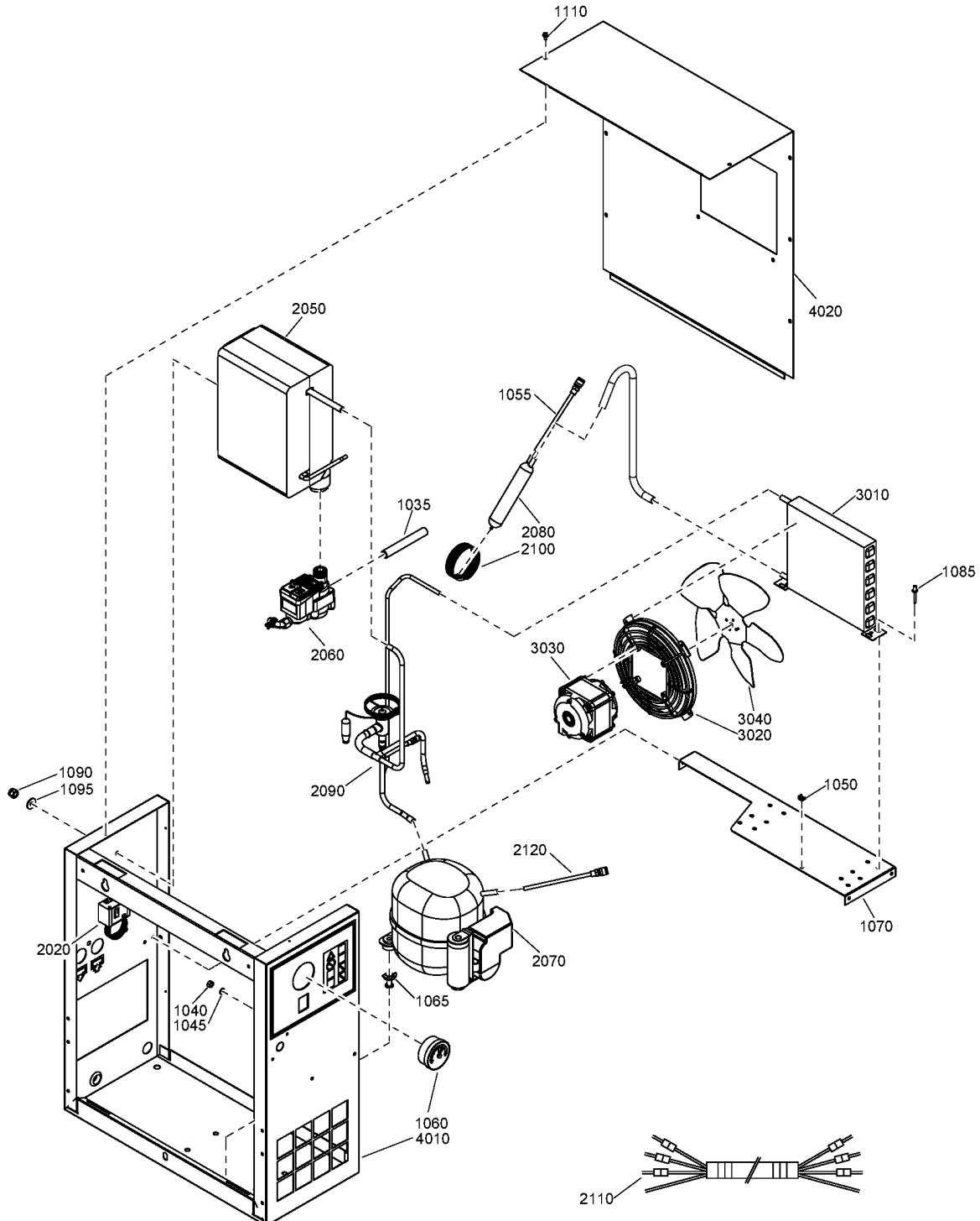
**21 - Air dryer components CPM 15, CPM 20 - (230V/50Hz - CE, 400V/50Hz - AS1210, CE, MOM, SAASME) - IEC - Without integrated dryer size, CPM 10 - 400V/50Hz - IEC - With 1 time size integrated dryer (08/11/2018 - ...)**
