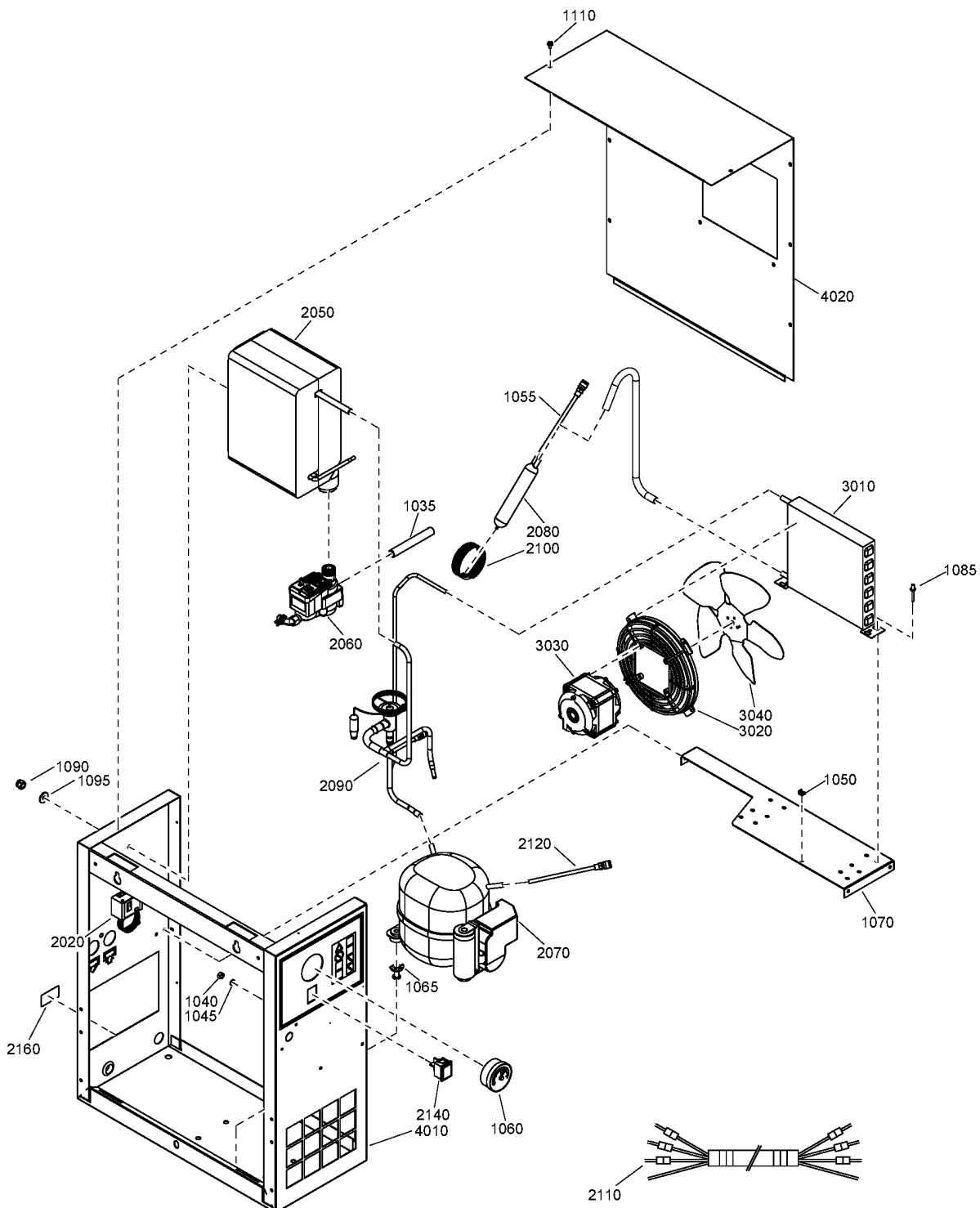
**29 - Air dryer components QRS 15, QRSM 20 - TRI-V/60Hz - ASME - UL-cUL -**
