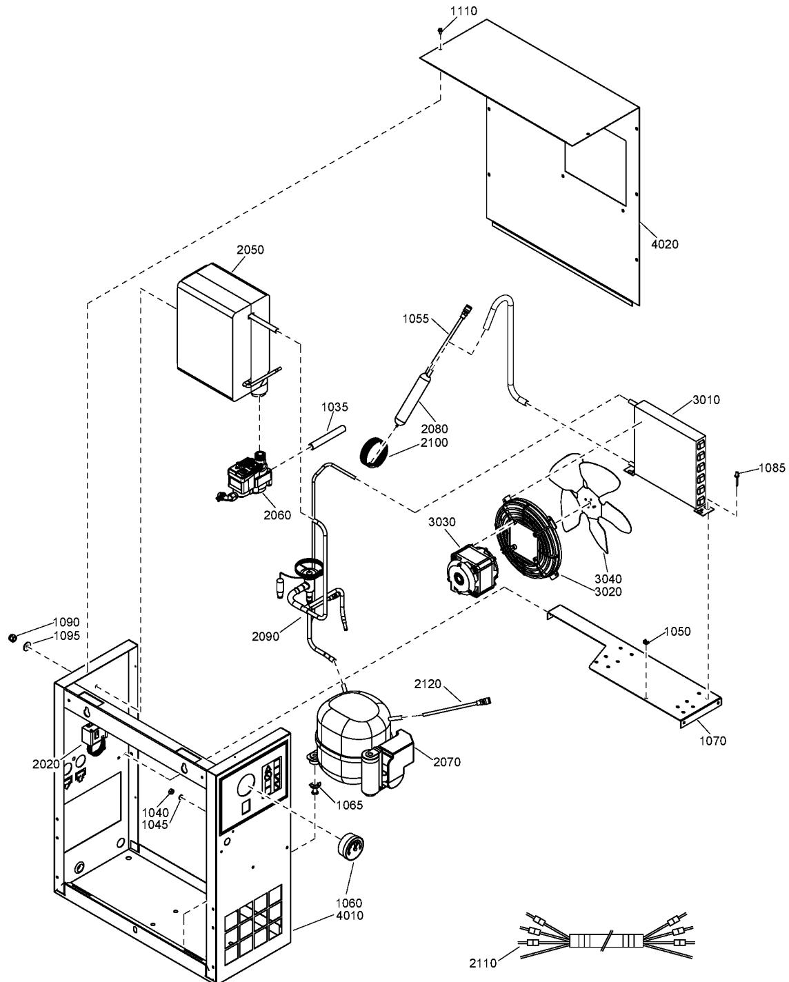
**25 - Air dryer components CPM 15, CPM 20 - 230-380-440V/60Hz - CE - IEC -**
