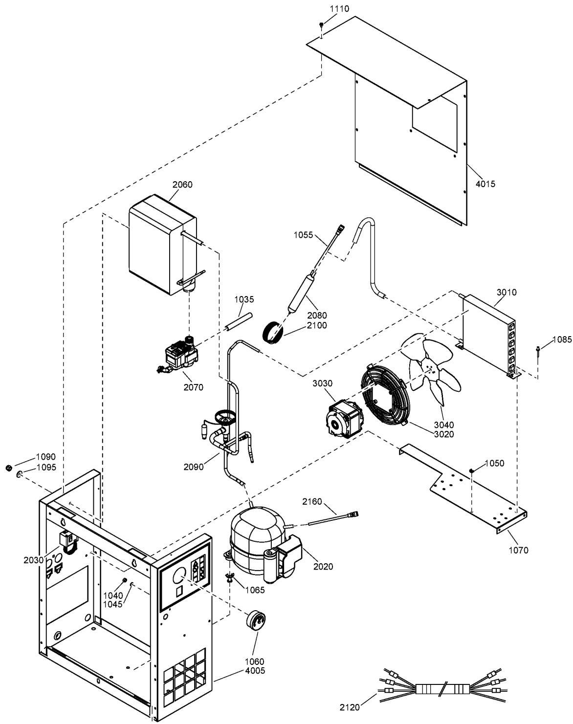
**23 - Air dryer components CPM 10 - 230V-380V-440V/60Hz - CE - IEC - Without size integrated dryer (08/11/2018 - ...)**
