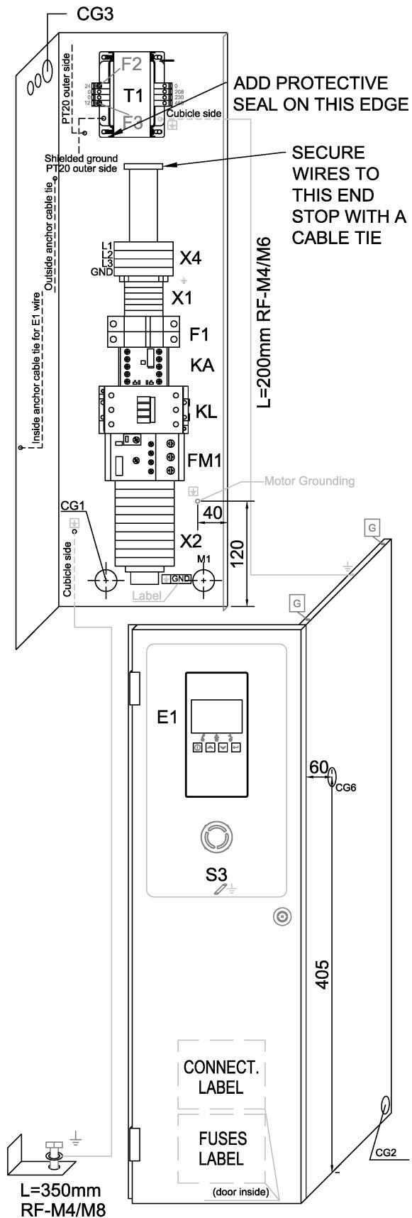
**47 - Cubicle components QRS 15 - Pack - 208-230-460V/60Hz - CSA/UL-cUL -
