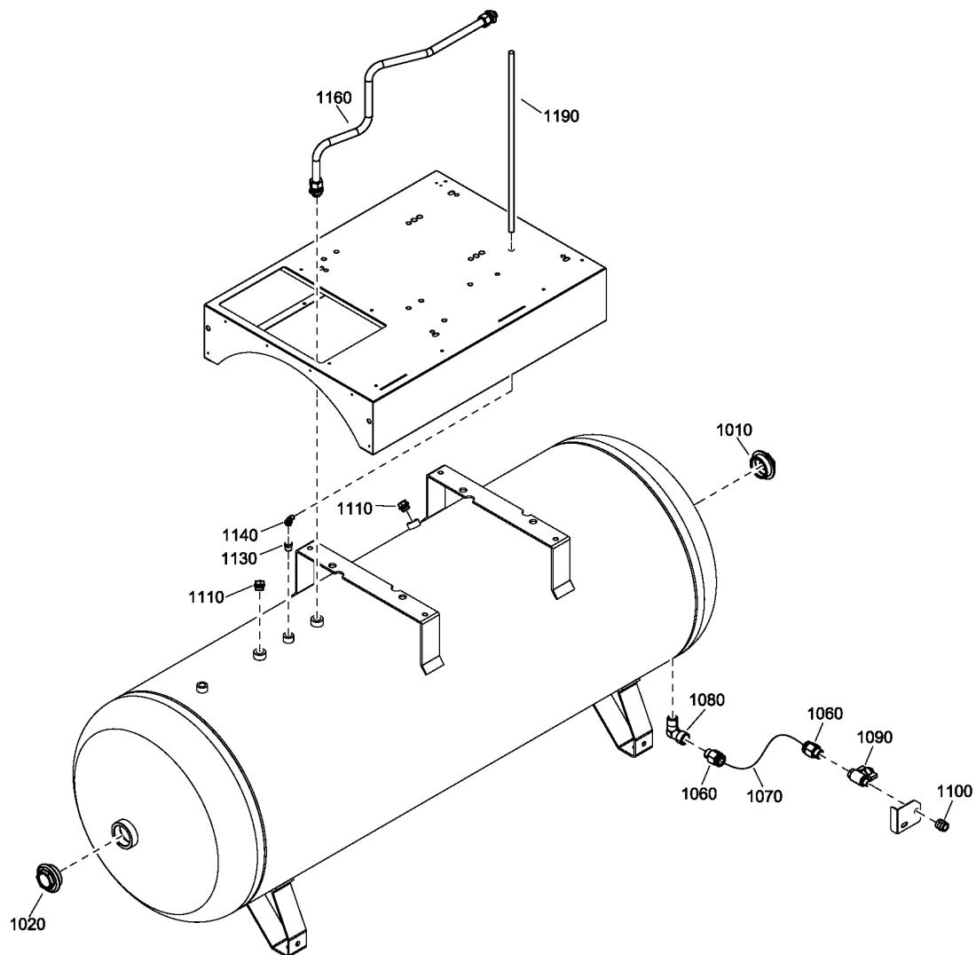
**14 - Air outlet CPM 10, CPM 15, CPM 20, QRS 10, QRS 15, QRS 20M - Pack - Tank
