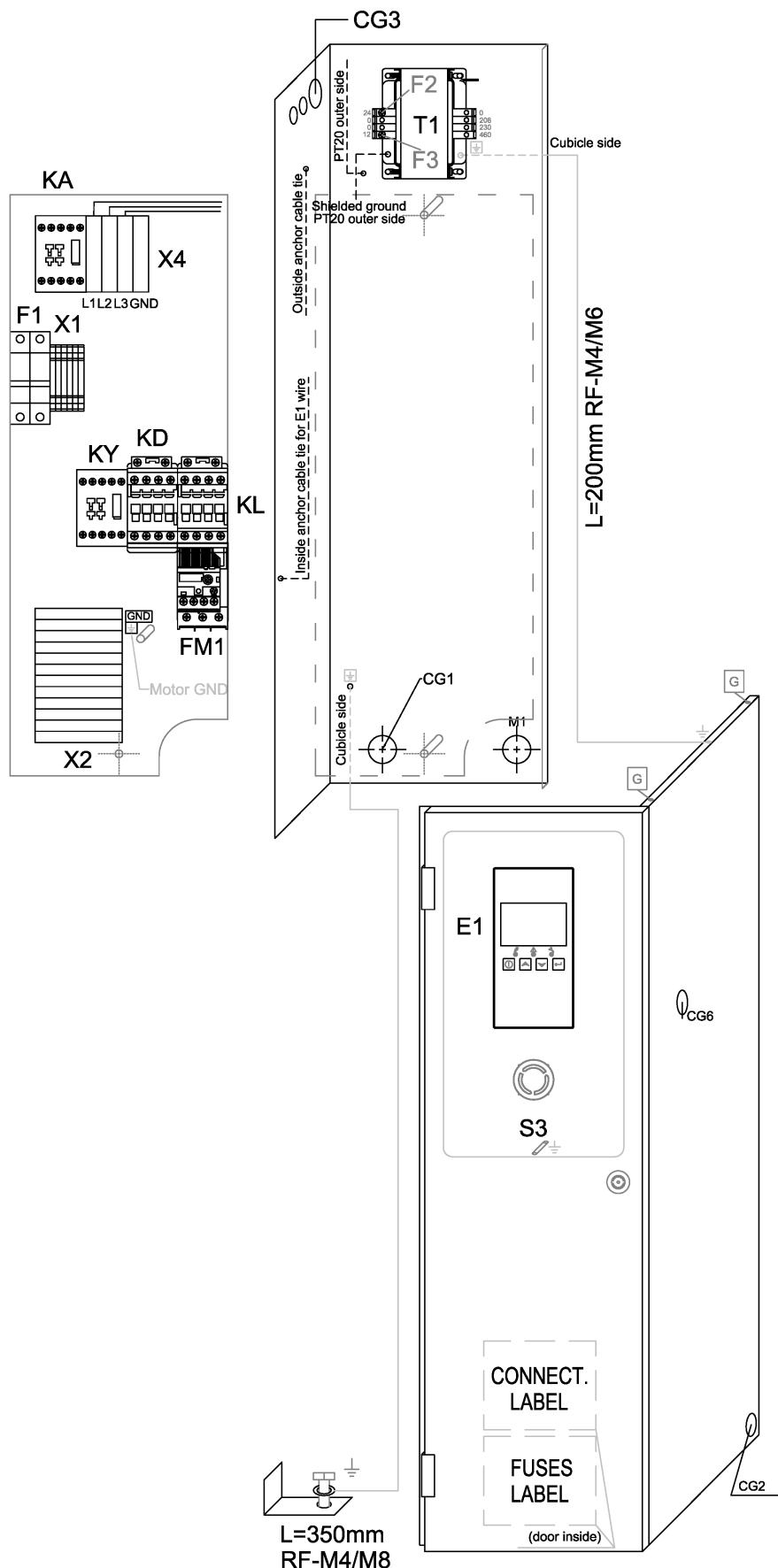
**48 - Cubicle components QRSM 20 - Pack - 208-230-460V/60Hz - CSA/UL-cUL -
