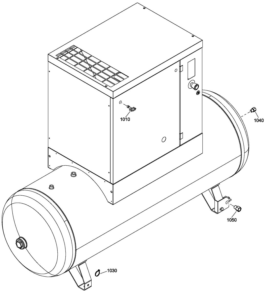
**73 - Loose parts CPM 10, CPM 15, CPM 20, QRS 10, QRS 15, QRSM 20 - Tank
