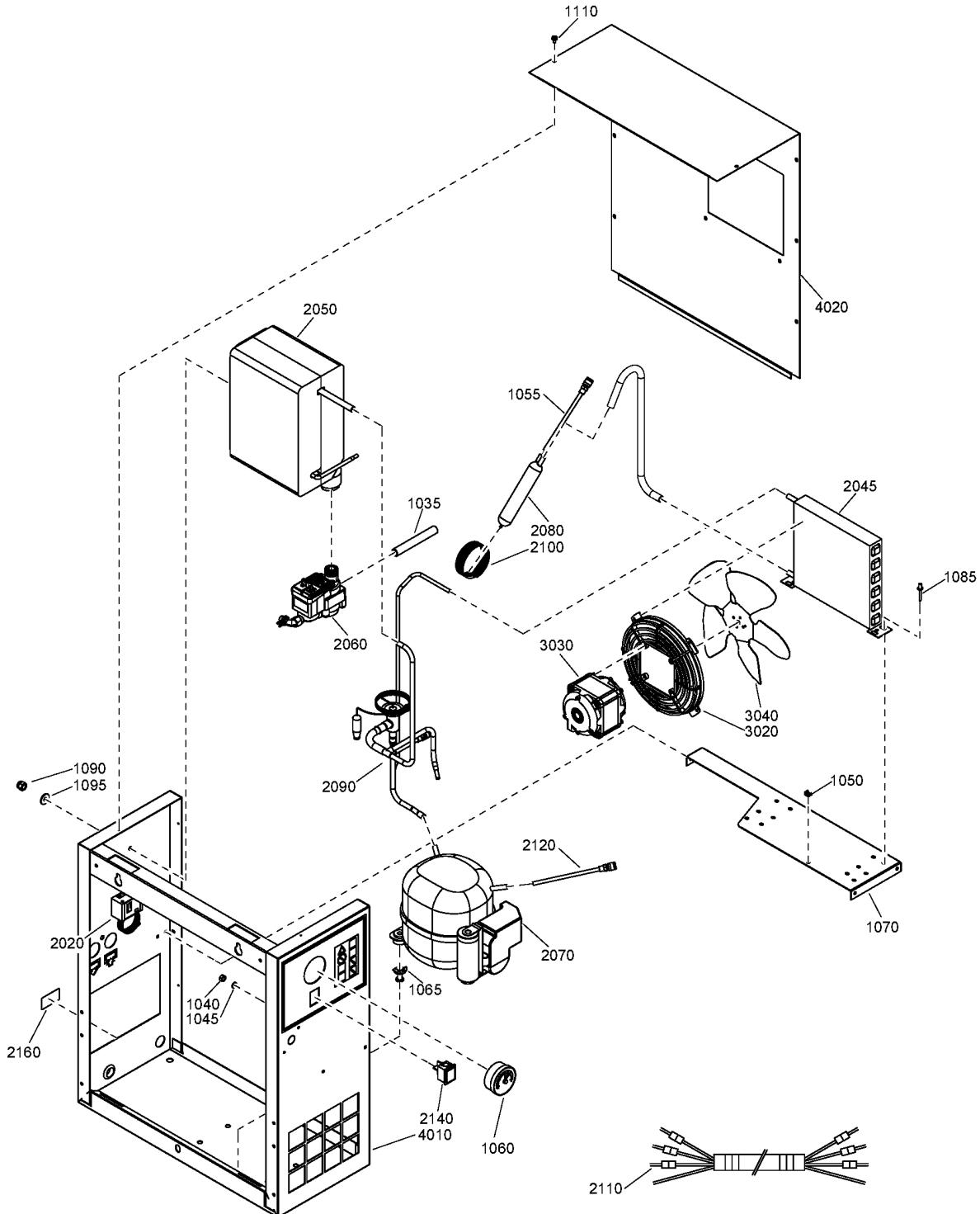
**31 - Air dryer components QRS 10 - TRI-V-575V/60Hz - CRNASME - UL-cUL -**
