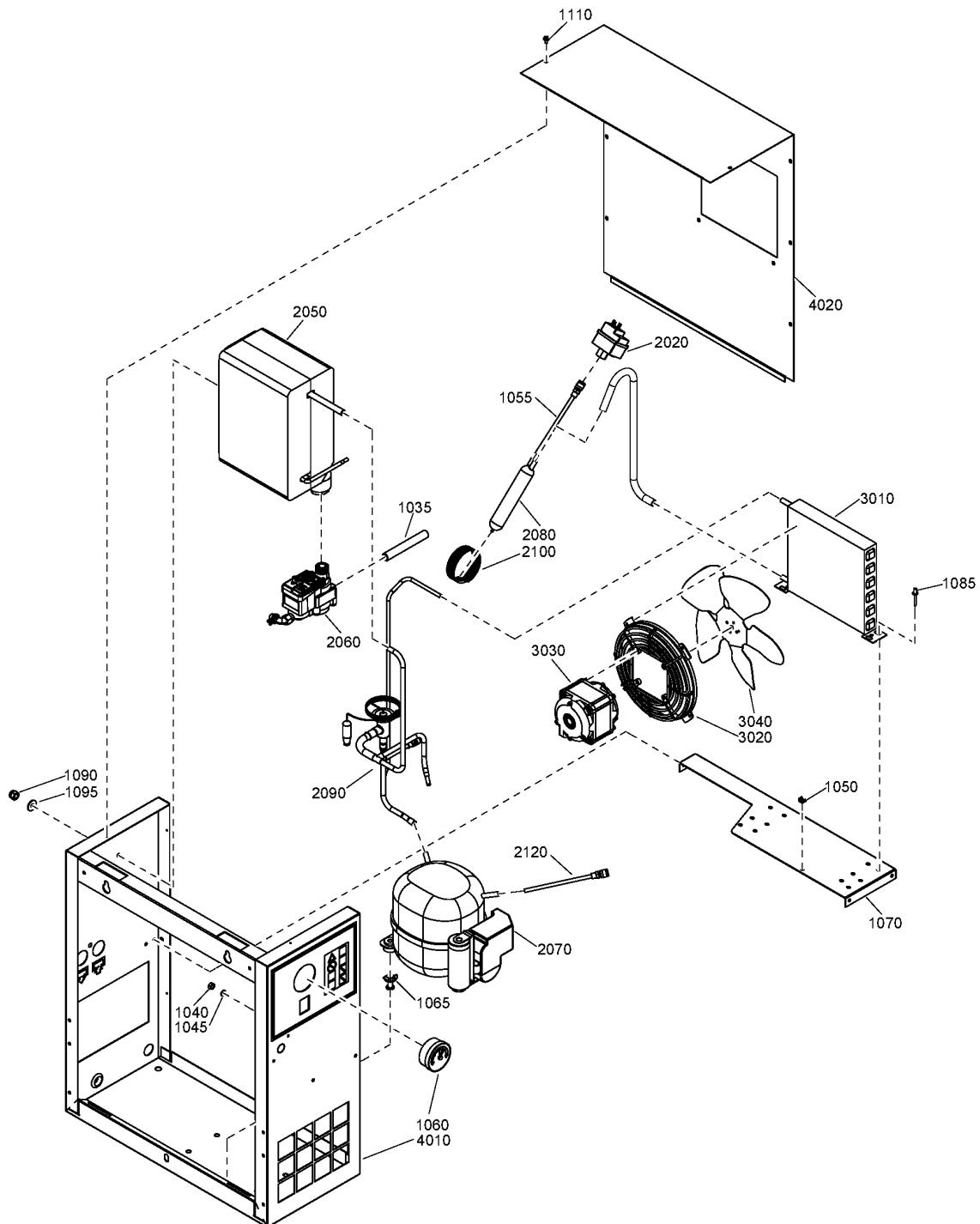
**24 - Air dryer components CPM 15, CPM 20 - 230-380-440V/60Hz - CE - IEC -**
