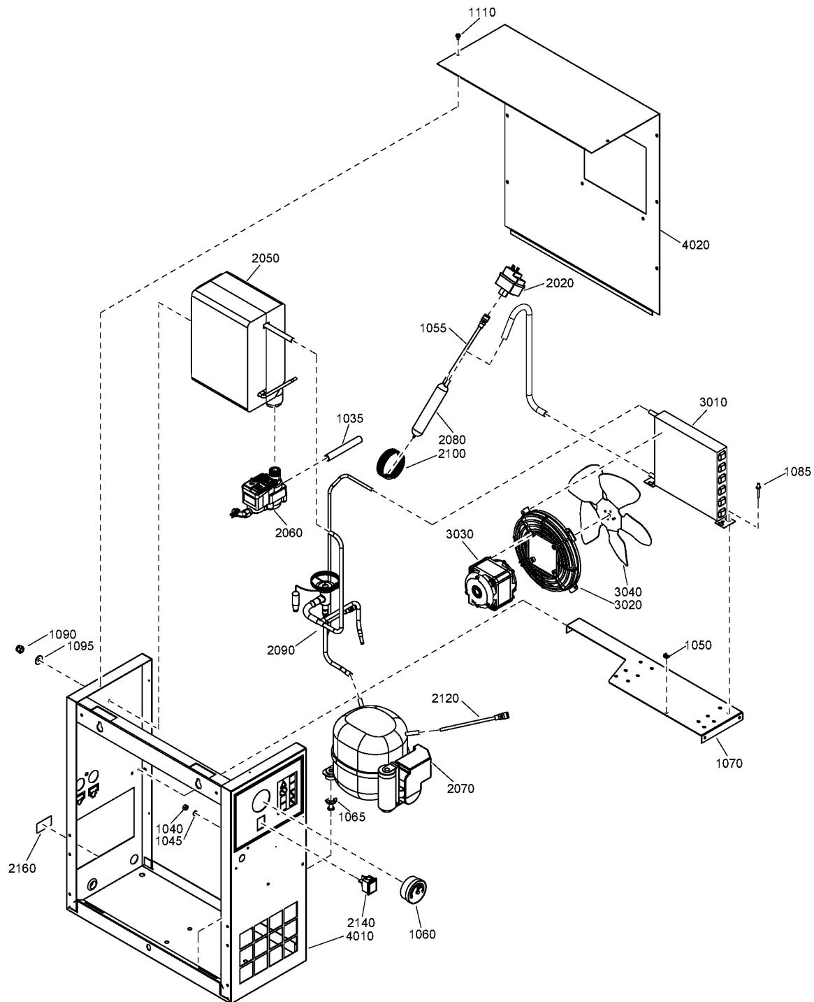
**28 - Air dryer components QRS 15, QRSM 20 - TRI-V/60Hz - ASME - UL-cUL -**
