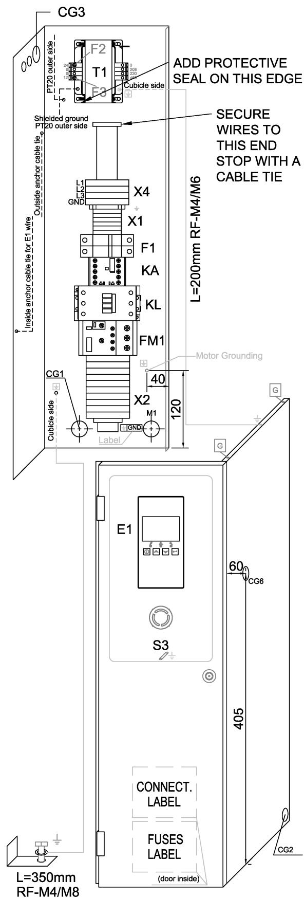
**46 - Cubicle components QRS 10 - Pack - 208-230-460V/60Hz - CSA/UL-cUL -
