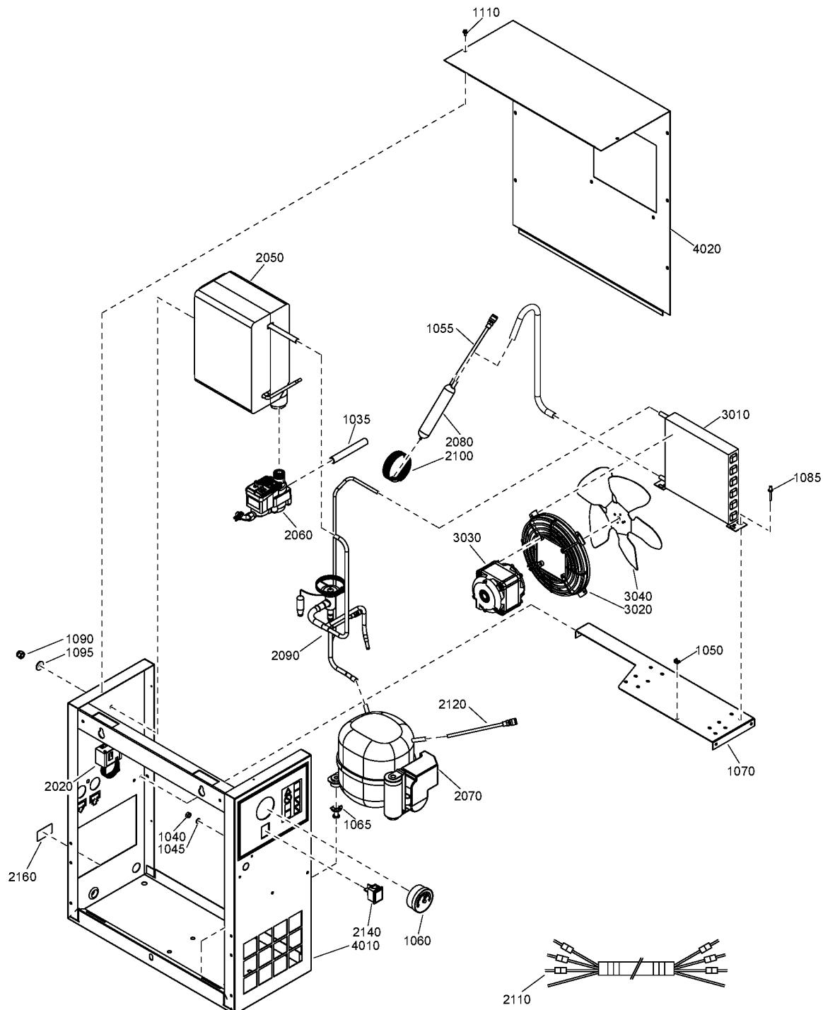
**27 - Air dryer components QRS 10 - TRI-V/60Hz - ASME - UL-cUL - Without size integrated dryer (28/09/2018 - ...)**
