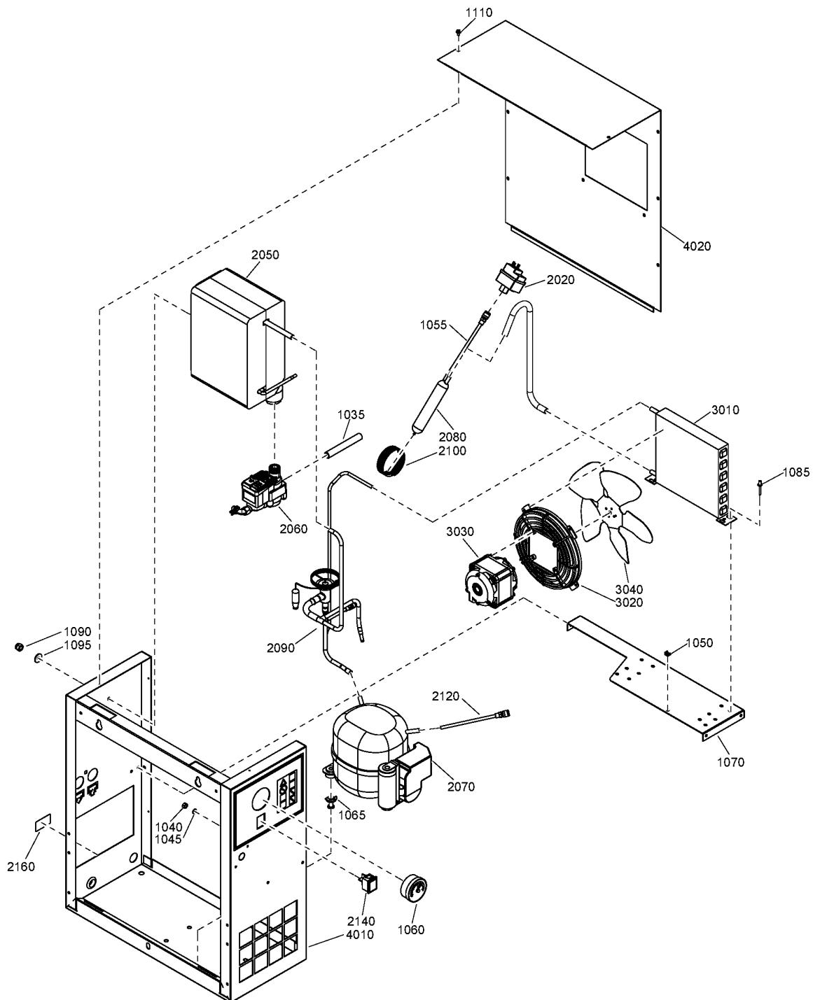
**26 - Air dryer components QRS 10 - TRI-V/60Hz - ASME - UL-cUL - Without size integrated dryer (11/10/2016 - 27/09/2018)**
