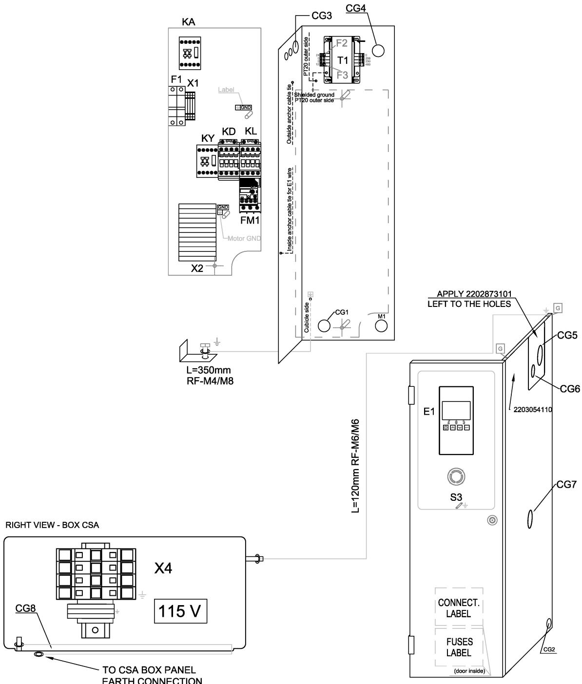
**51 - Cubicle components QRSM 20 - Full-Feature - 208-230-460V/60Hz - CSA/UL-cUL - CRNASME**
