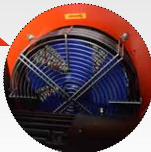
**6. RADIATOR/COOLING FAN/MOISTURE SEPARATOR**
