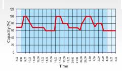
**Profile 3:** this profile represent an application with an eight-hour shift at constant consumption for five days a week. Air demand tends to stay around 90% of maximum requirement.
