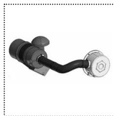
The **high efficiency intake filter** is able to hold solid particles of more or equal to 3 micron with a filtering efficiency of 99%.
