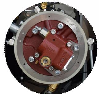
**7. HYDRAULICALLY CONTROLLED AIR INLET VALVE**
