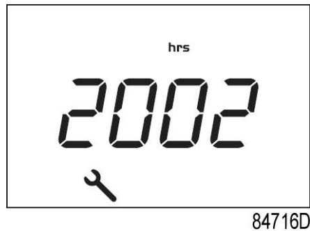
Example of running hours screen
