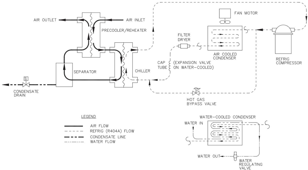
Figure 1 - Flow Diagram
