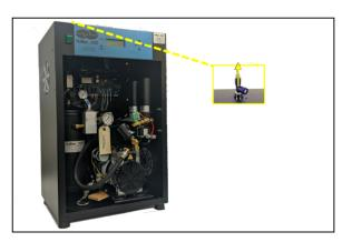
6.5.7 Install the Plug into the included Precision BleedOrifice Fitting and then into the dryer Outlet Port.
