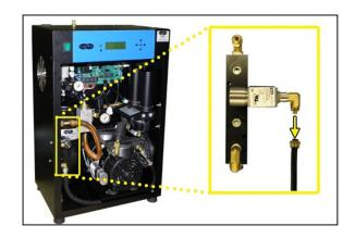
**9.7.4** Place your hand under the Unloader Valve to verify for air flow.
