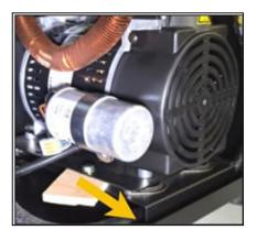
**6.5.6** Remove the Plug from the Outlet Port by pressing the ferrule down then pulling the plug upward.
