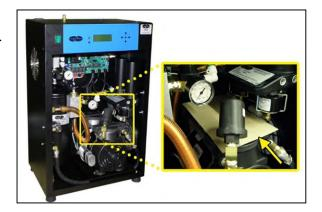
9.6.3 Locate the heatless dryer purge solenoids inside the air dryer.
