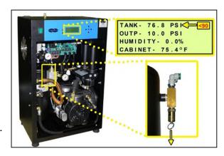
When the Compressor runs for 3:00 minutes (unless adjusted to a different Set Point by the user), a High Compressor Last Run Time (LAST RUN) alarm should appear on the System Screen.
