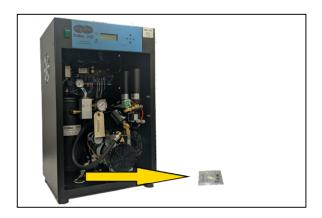
**6.5.5** Remove the wooden shipping block from underneath the compressor.
