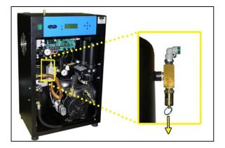
If the Safety Relief Valve fails either test described, it must be replaced. See sections 11.2 for part detail and 11.7 for ordering information.
