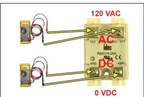
**9.5.6** Use a Voltmeter to measure across the DC terminals. Should measure **0 VDC**.
