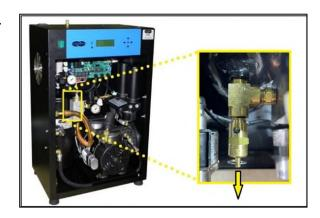
9.13.4 Unscrew and remove the Humidity Sensor from the Humidity Block.
